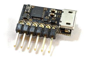
It features the Silicon Labs CP2102N chip for excellent cross platform driver support, on-board autoprogram circuitry to transparently handle device programming and serial console use, a V+ blocking diode and ESD protection. The pull-up resistors for IO0 and EN are not on this module, they are on the wESP32™ since they have to be present to correctly boot and run the ESP32 if the programming submodule is not present.
